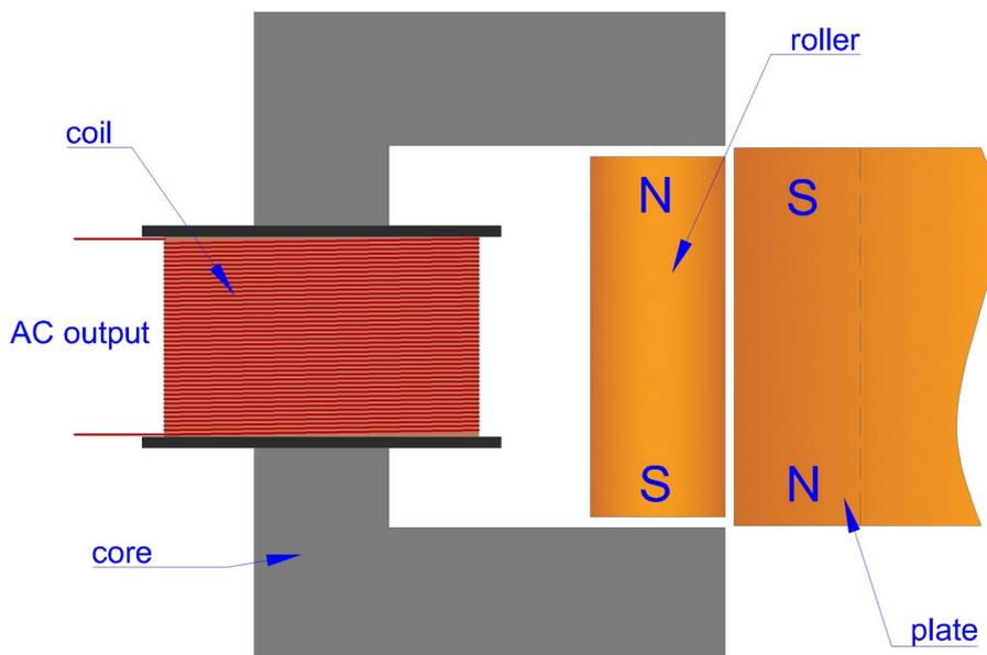
Figure 5: Roller inside ferromagnetic core gap.
