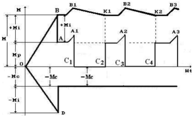
Fig. 11. Diagram of the change of the torques, which act on the rotor at the time of its start and during uniform rotation
