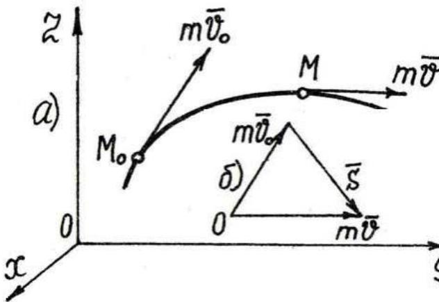
Fig.1. Diagram to a determination of action of force  $\vec{S}$
