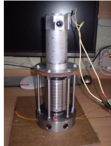
Fig. 10. Electromechanical generator of electric pulses
