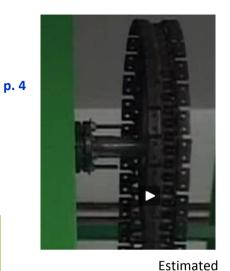
733.46 Nm  $P_a = 2*\pi*M*n$ 0.154 kW corresponding to Rosch P<sub>in</sub> = 0.149 kW 3% loss 5th line
